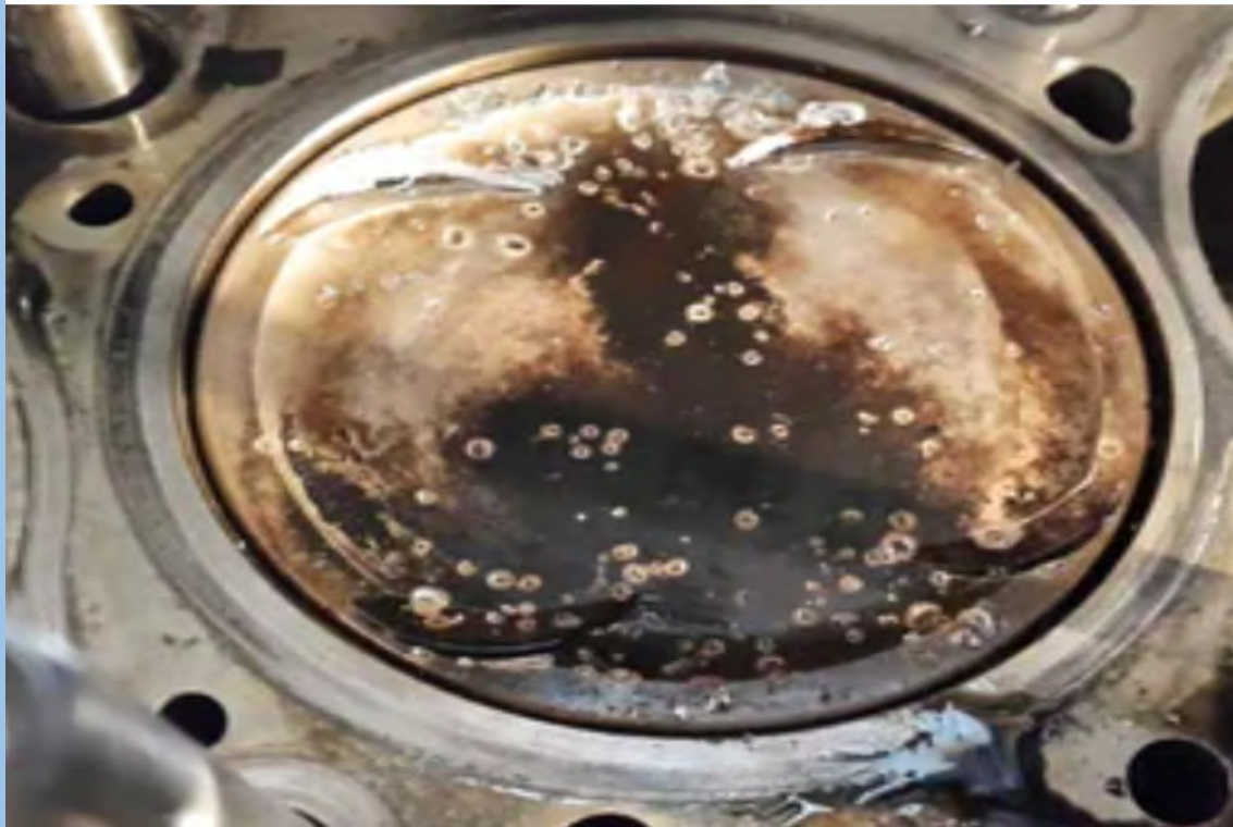
Detonation damage to Piston
