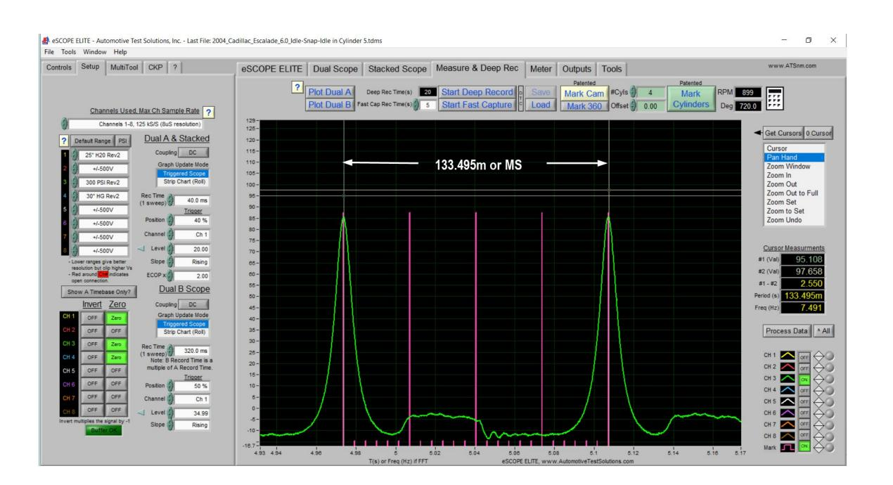
I prefer to capture about 8 seconds of cranking compression to get a meaningful capture.
