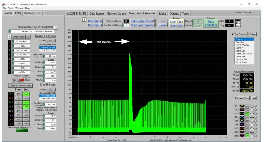
An engine cranking at 145 rpm completes a single 720° revolution in about 830.5 Milliseconds.
