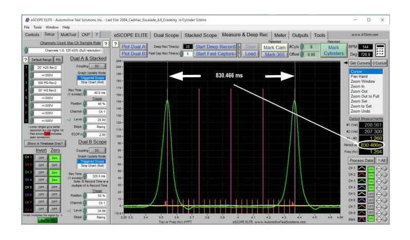
Start thinking about an engine idling at say 900 rpm or a snap throttle of 3650 rpm and the same 720° rotation takes 133.524 ms. and 32.909 ms. respectively.
