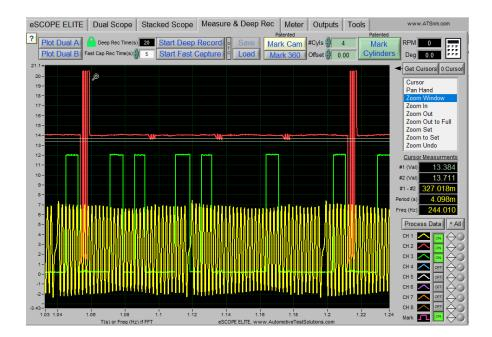
Start thinking about how fast events happen on a running engine and you will begin to understand the correct sweep times for the data you are using to diagnose.
