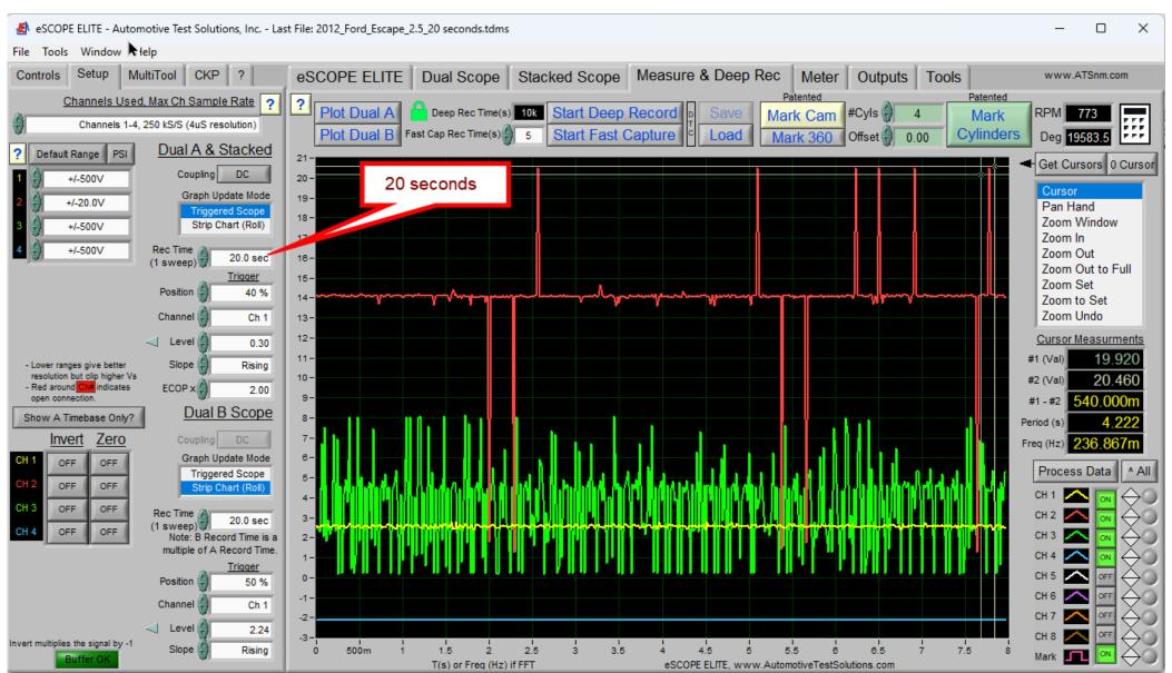
Here is the 20 second sweep time capture zoomed in, no useful data here at all. 20 seconds of sweep time is way to slow and equates to 2.77 hours of total capture time.
