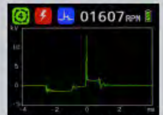
Displays secondary ignition waveforms.
