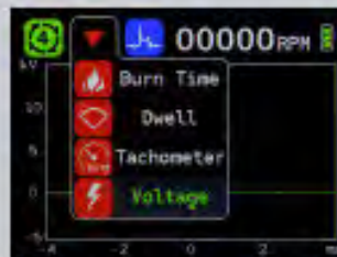
Displays and measures spark burn (firing) time, dwell time, current ramp time, RPM, and spark plug peak voltage.
