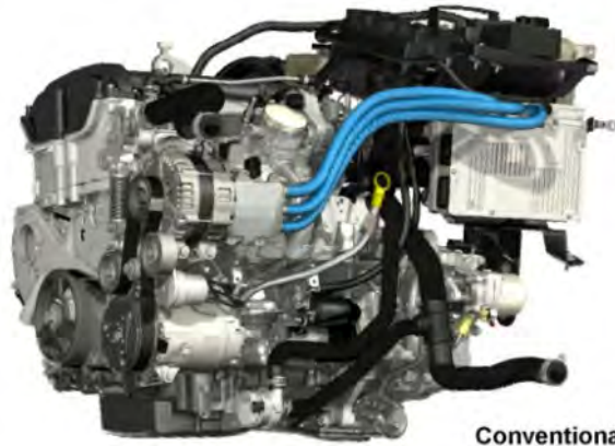
Conventional Engine with a Generator with Starter
