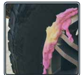
BULLSEYE Leak Detector Quickly finds wheel and tire problems.
