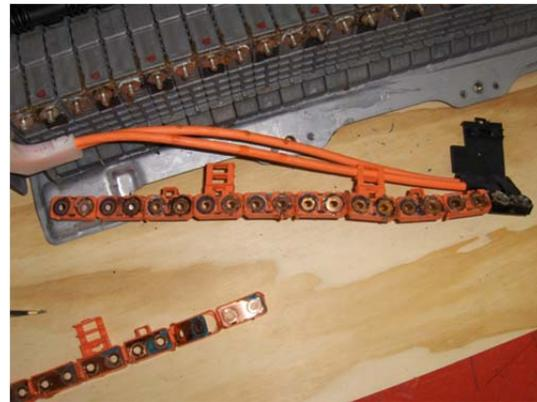
Now just changing cells is not going to cut it since we still had the corroded copper bus bar connectors. To clean up the copper bus bars you
