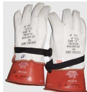
battery always has power, just like a flash light even when the switch is off the batteries (if good) still have voltage. Make sure to check the HV gloves covers (outer leather covers) for any cuts or holes flowed by checking the HV gloves for pinholes by using the roll up test (capture air in the glove while rolling it up). In my opinion if you think the glove has been compromised send it out to be professional test rather than risking it.
